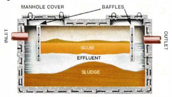
All household waste is disposed of through the septic system. The proper operation of the septic is essential to health, property value, and the ecology. A small commitment to the care of your septic system will protect you from the nightmare created by a failing system.
